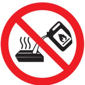
**It is forbidden to refill biofuel while the device is operating.
