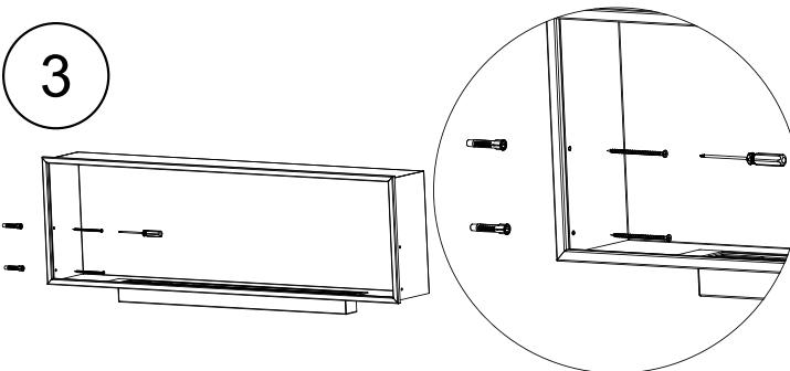
If the bioethanol fireplace is already attached to a niche, we use the existing mounting holes (do not punch new ones). The glass holders and fastening of the bioethanol fireplace are done simultaneously in one step. Attach the glass holders using the screws and dowels supplied with the bioethanol fireplace.
