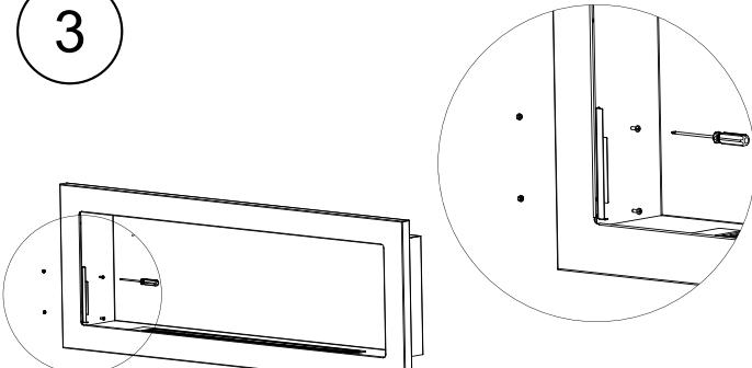
The glass holders should be fixed using the screws and nuts included in the kit.
