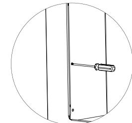
The mounting points closer to the front frame of the bioethanol fireplace should be removed with e.g. a screwdriver or other tool by pressing in.
