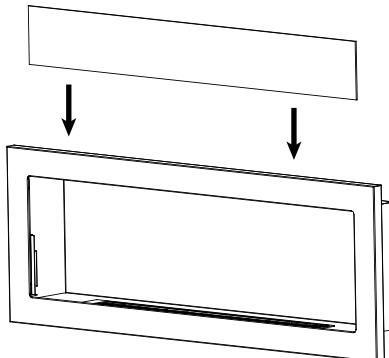
Slide the glass into the holders from top to bottom.
