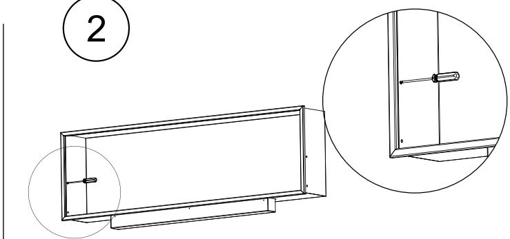
The mounting points closer to the front frame of the bioethanol fireplace should be removed with e.g. a screwdriver or other tool by pressing in.
